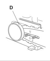
2 The front hand guard is not designed solely to activate the chain brake. Another important safety feature is that it prevents the chain from hitting your left hand if you lose your grip on the front handle.
